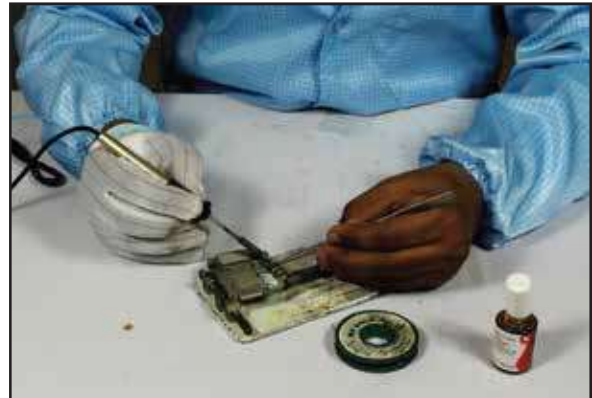
Fig: 3.2.5.5 Charging Connector Soldering - Step 2
