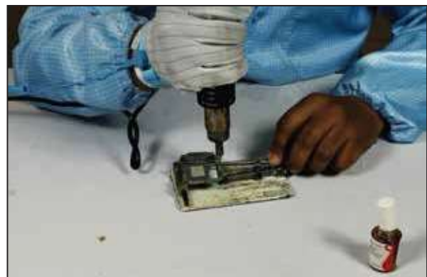
Fig: 3.2.5.2 Soldering Flux on Charging Connector
