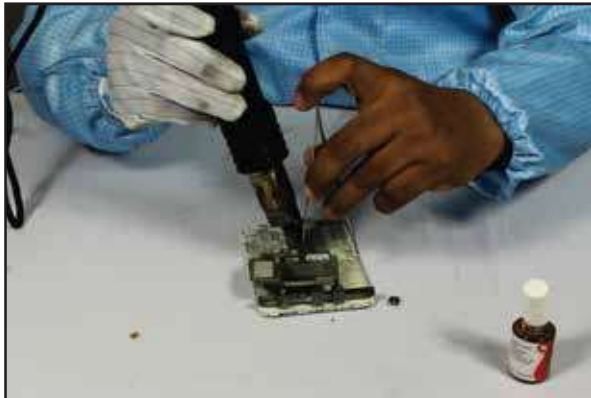
Fig: 3.2.5.4 Charging Connector Soldering - Step 1
