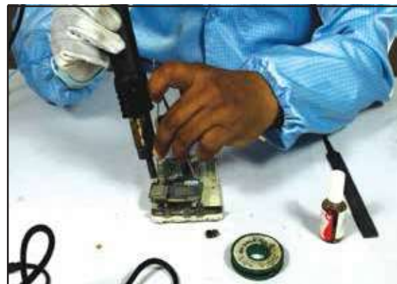
Fig: 3.2.5.9 Headphone Connector Soldering - Step 2
