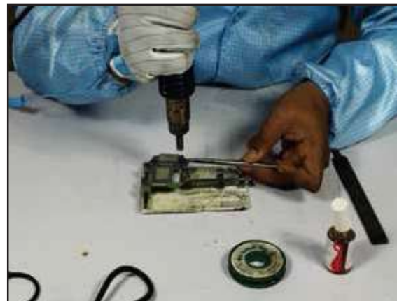
Fig: 3.2.5.8 Headphone Connector Soldering - Step 1
